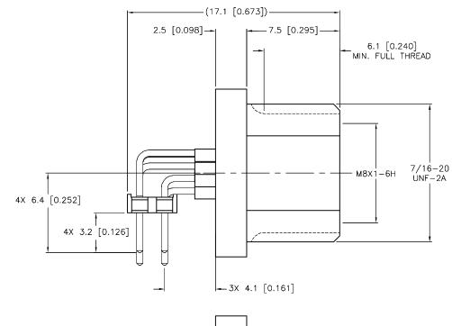
1. "/CS10712" DESIGNATES RECEPTACLE WITHOUT O-RING AND LOCKNUT.
